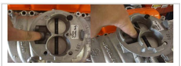
If you have a scanner, adjust the IAC count at idle to be between 40-60 counts. You can also install a false IAC sensor in the plug to fool the PCM into believing there is a idle control when you are setting the idle by the throttle plates directly, the false sensor will operate while the original IAC motor sits idle in the throttle body. This eliminates the long decel times after rev'ing the throttle.
