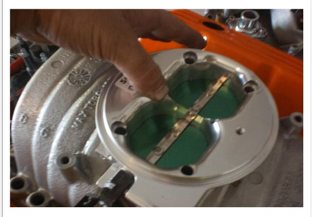
This is a picture of a Flometrics 58mm throttle body IAC being plugged for throttle adjust while idling around 750-800 rpm.
