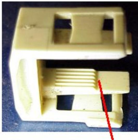
Here's a different view that better shows the inner locking teeth that keep the cable in position
