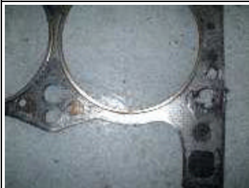
(3) Driver-Side Head Gasket: #4 (Notice the fire ring at the top of the cylinder - ring partially distorted due to misaligned o-ring)
