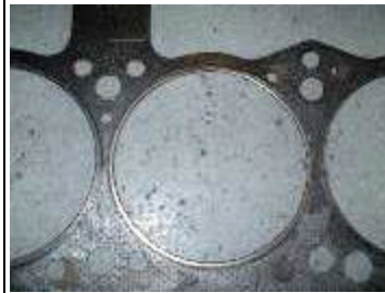
(2) Passenger-Side Head Gasket: #2 Cylinder (Notice misaligned O-Ring and partially crushed fire-ring due to misalignment of O-Ring)
